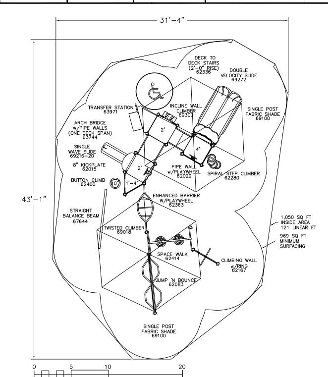
It is the manufacturer's opinion that the structure shown herein complies with current ada standards concerning accessibility if used with proper accessible surfacing and together with other necessary ground level play equipment.
