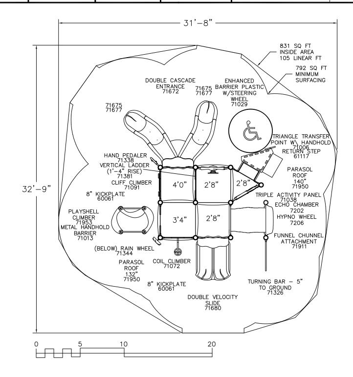
It is the manufacturer's opinion that the structure shown herein complies with current ada standards concerning accessibility if used with proper accessible surfacing and together with other necessary ground level play equipment.
