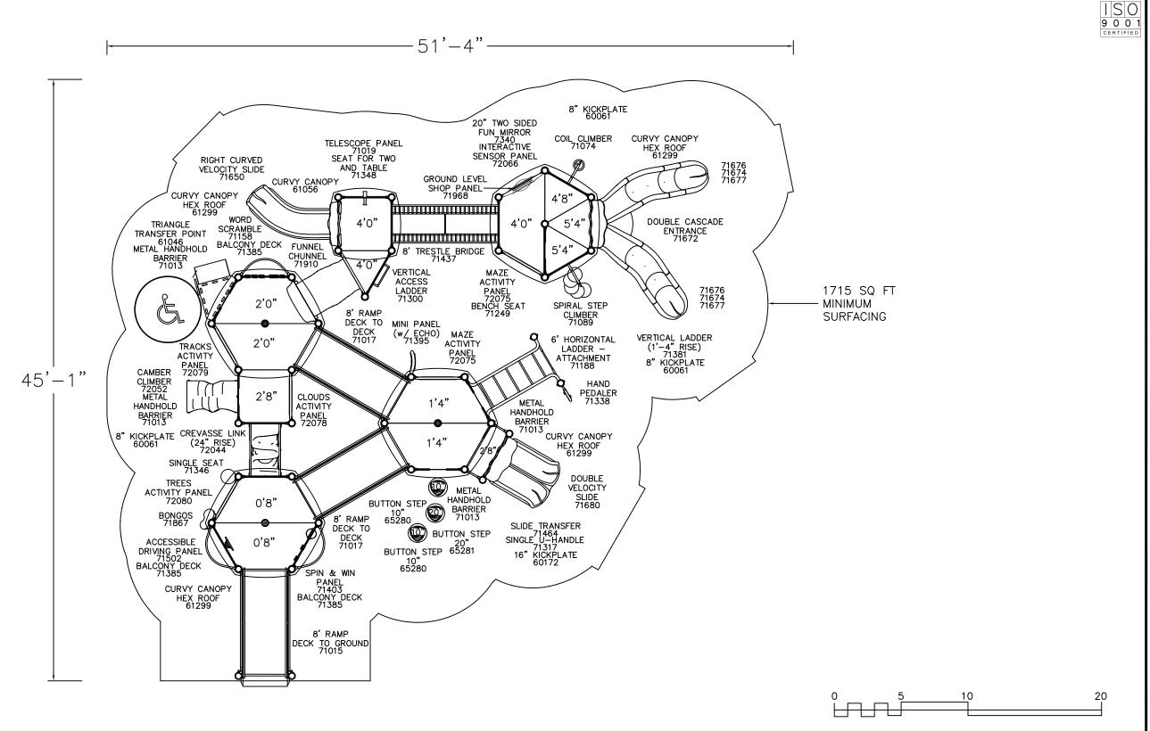
It is the manufacturer's opinion that the structure shown herein complies with current ada standards concerning accessibility if used with proper accessible surfacing and together with other necessary ground level play equipment.
