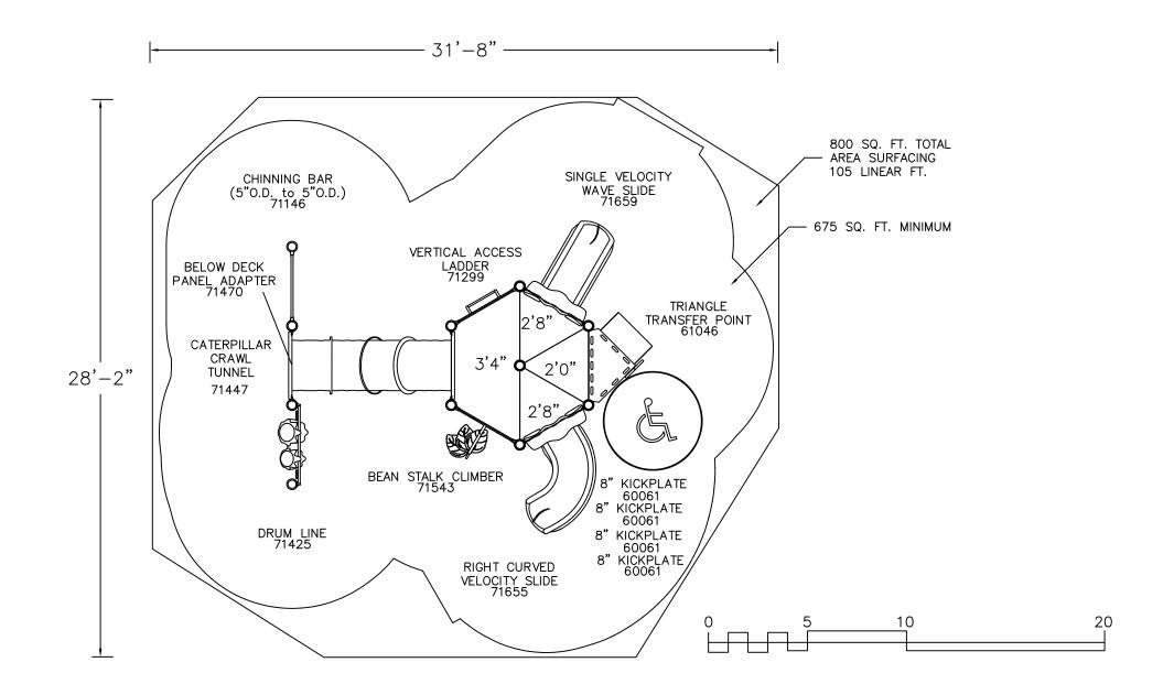
It is the manufacturer's opinion that the structure shown herein complies with current ada standards concerning accessibility if used with proper accessible surfacing and together with other necessary ground level play equipment.
