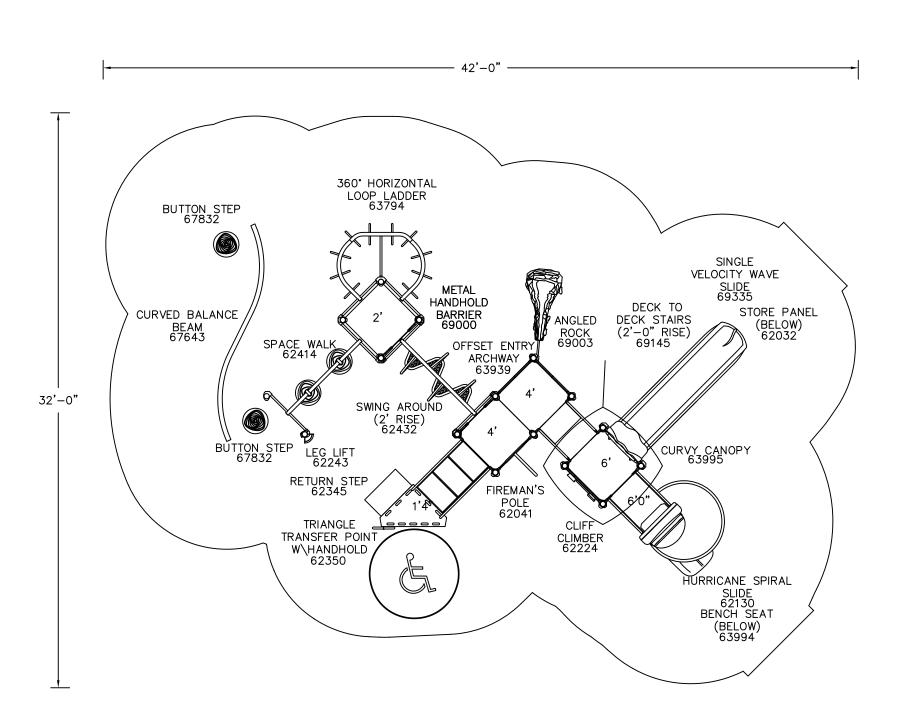
It is the manufacturer's opinion that the structure shown herein complies with current ada standards concerning accessibility if used with proper accessible surfacing and together with other necessary ground level play equipment.
