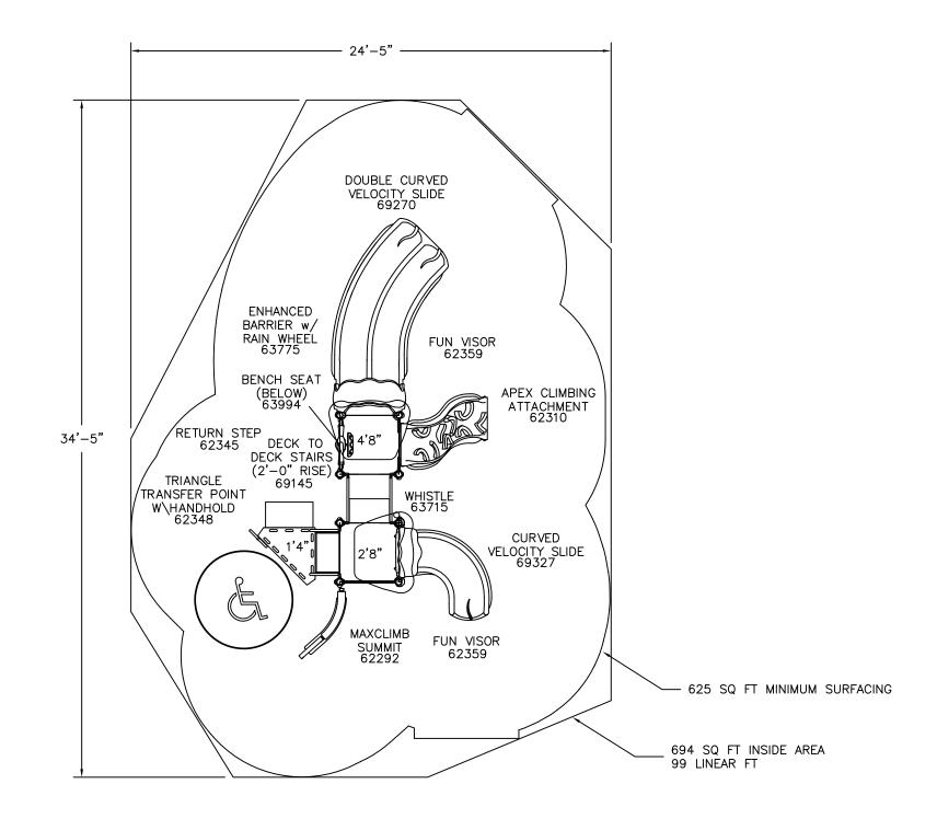
It is the manufacturer's opinion that the structure shown herein complies with current ada standards concerning accessibility if used with proper accessible surfacing and together with other necessary ground level play equipment.
